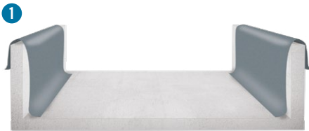
1 Install RaniSidewall film
